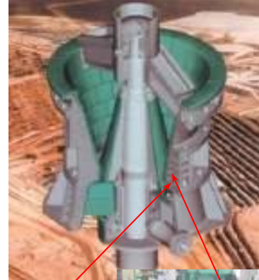
Cladding of Crusher - Increased life
