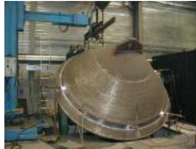
Cladding of Crusher - Increased life
